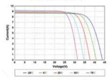
Current-Voltage Curves at Different Temperatures
